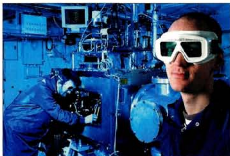
Alec Thomas (left) and Stuart Mangles (right) of Imperial College London with the Astra laser used at the Rutherford Appleton Lab in work on laser wakefield acceleration.
