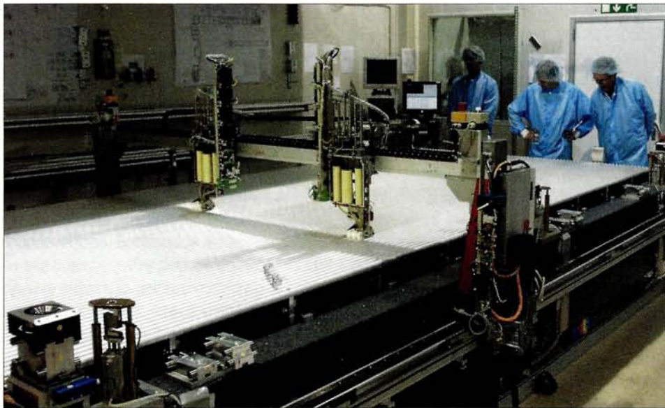
Assembly of a complete muon chamber for the outer layer of the ATLAS barrel muon system.
